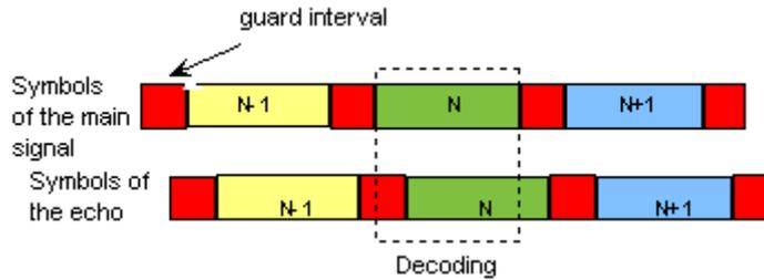
You have to reduce the level of reception of the echoes by orienting the antenna or by selecting a more directive antenna.
