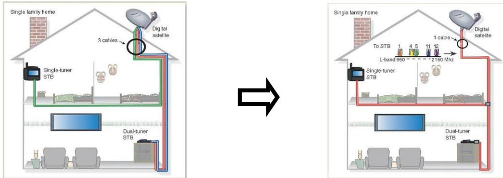
The DCSS is an extension of the DiSEqC protocol that allows the connection of several receptors on **only one coaxial cable**, no matter the band (H/L) and the polarization (H/V).
