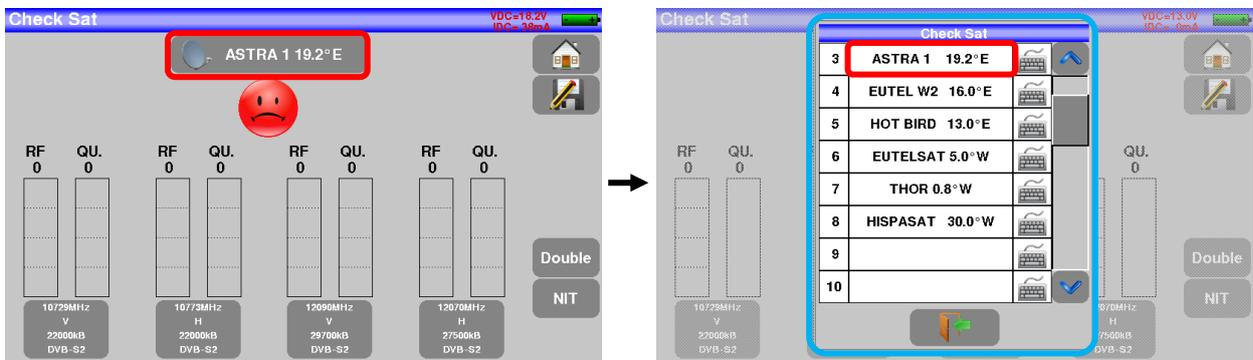
→ The device successively scans 4 transponders and gives an RF indication corresponding to the level of the signal received on the antenna and QUALITY corresponding to the quality of the signal received on the antenna.
