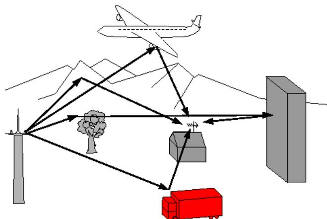
In digital TV DVB-T/T2, these echoes may help or degrade the image according to the time delay between the various signals that reach the antenna.
