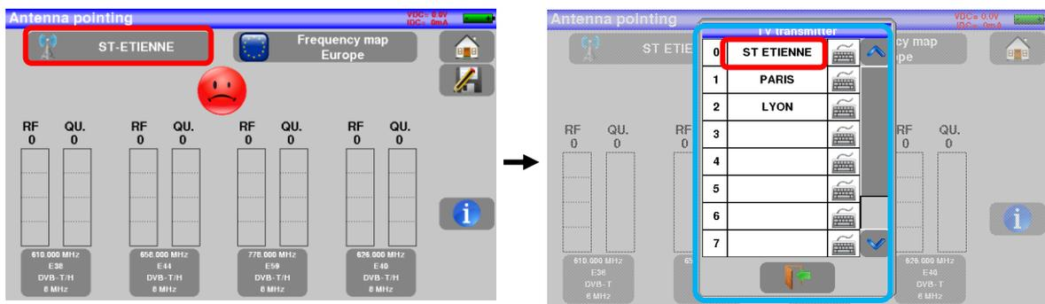
→ The device successively scans 4 channels and gives an RF indication corresponding to the level of the signal received on the antenna and QUALITY corresponding to the quality of the signal received on the antenna.
