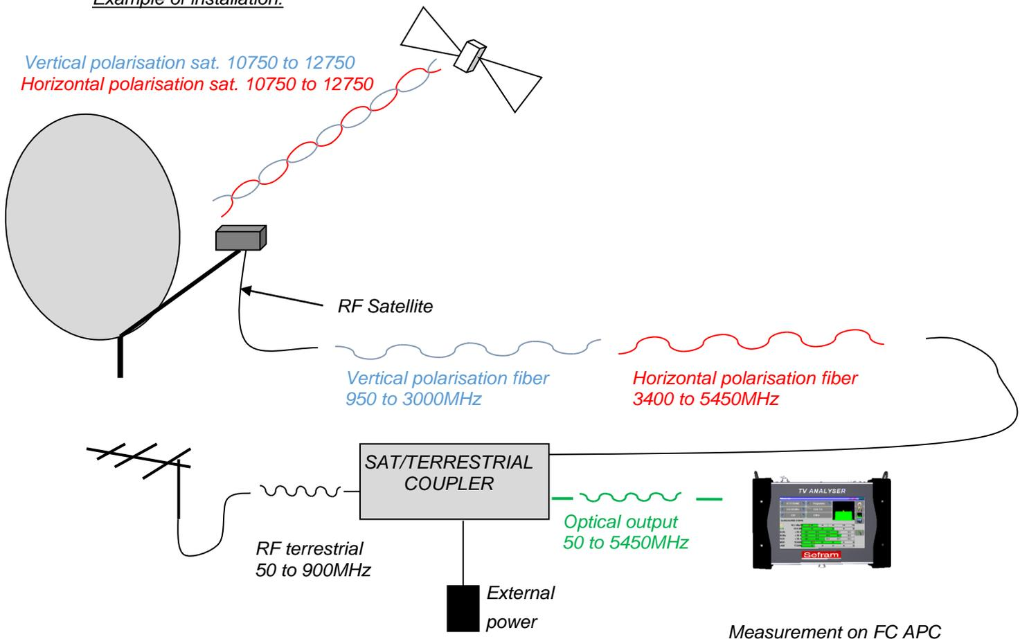
To display the signal at the output of your installation, you must connect the RF output of the optical option to the RF input of the appliance via the provided angled F/F cable. Power your coupler (no external power supply is provided with the measurement appliance).
