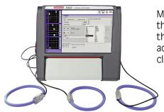
Measurements are done with the voltage input (direct) of the universal board and accessories clamps (standard clamps or flexible clamps)
