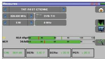
All measurements are displayed with a clear color set: green if measurement is OK, red if measurement is off limits.
