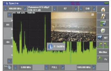
A zoom function is provided to check in detail TV signals and the quality of the TV installation.
