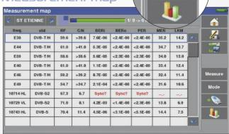
Select the frequencies you want to monitor: all measurements will be recorded with timestamped information. Your records can be transferred on USB memory stick. Files (.csv) can be read and used with Excel™.
